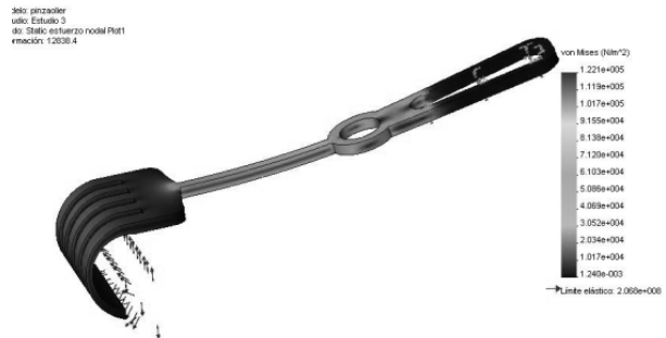
Figura 10. Tensiones en Pinza Ollier. Figure 10. Tensions in clip Ollier
