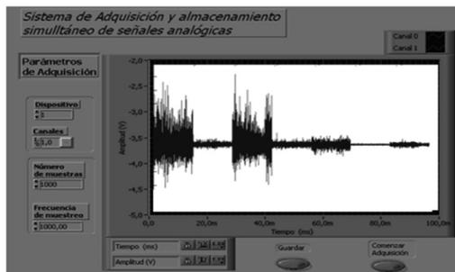
Figure 6. Electromyograph front panel
