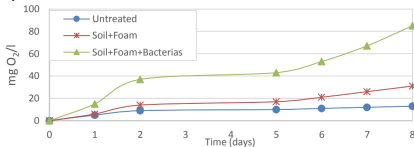
Figure 2. Degradation test results with spirometer (T.Vogel)
