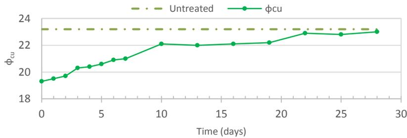
Figure 9. Evolution of the internal friction angle over the time
