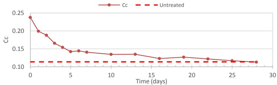
Figure 8. Evolution of the compressibility coefficient over time
