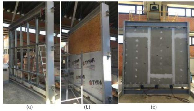
Figure 2. Sample-mounting sequence: (a) board with steel frames, (b) system enclosure (c) sample coupled to the furnace
