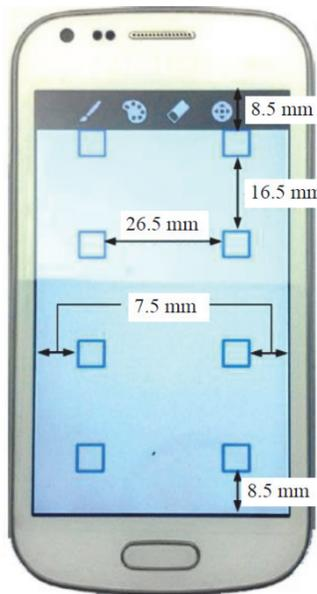
Figure 1. Position of targets on mobile phone screen.
