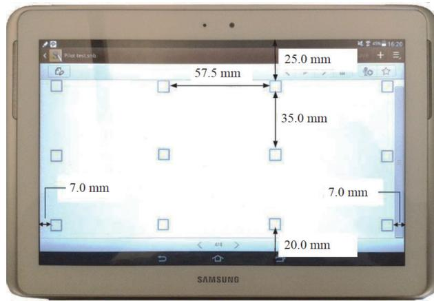
Figure 2. Position of targets on tablet screen.
